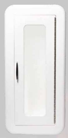
SPECIFICATIONS: Fire Extinguisher Cabinet, as manufactured by Cato, Inc., with body, bezel and door, injection molded of white virgin 2 Izod Co-Polymer Polypropylene of .15 wall thickness, virgin acrylic Plaskolite panel of .080 thickness, stainless steel hinge, chromium-plated door handle and roller catch.
